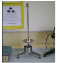
Plate 5: Torsion Viscometer
