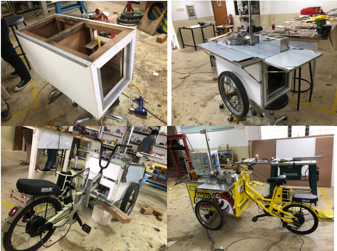
Figure 9: Upgrading process of the cart (Source: Author)
