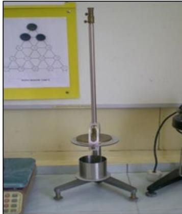
Plate 5: Torsion Viscometer
