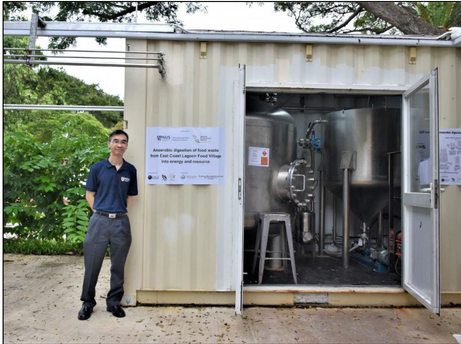
Figure 4 Associate Professor Tong Yen Wah, who leads the NUS team, is pictured next to the anaerobic digester at the East Coast Lagoon Food Village. (Source: News@NUS, 2024).
