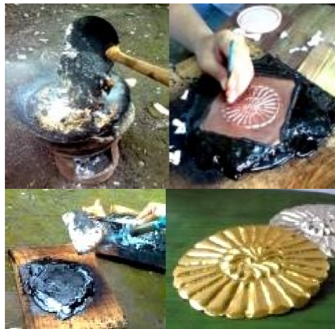
Figure 9: Chasing & Repoussé Process (Source: private collection, 2010)
