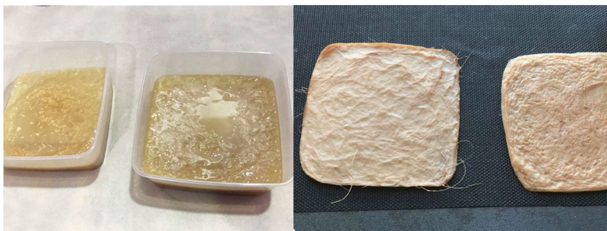
Figure 4: Bacterial cellulose in growth medium (left) and sun-drying and texture imprinted process (right)
